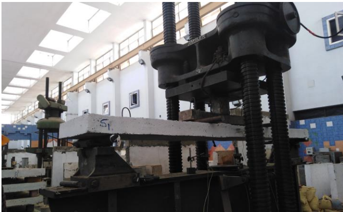
Photo 1: Test Setup of Slabs
