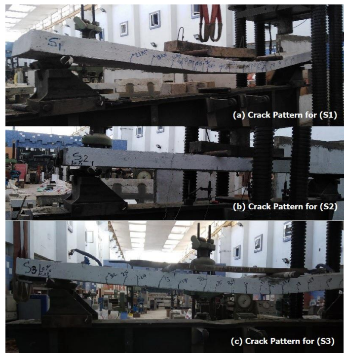
Photo 2: Crack Pattern for different Specimens
